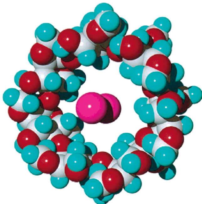
Figure 15. Illustration of the iodine molecule ( I_2 ) encapsulated by heptakis(2,6-di- O -methyl)- \beta -CD ( I_2 :DM \beta -CD). 193
